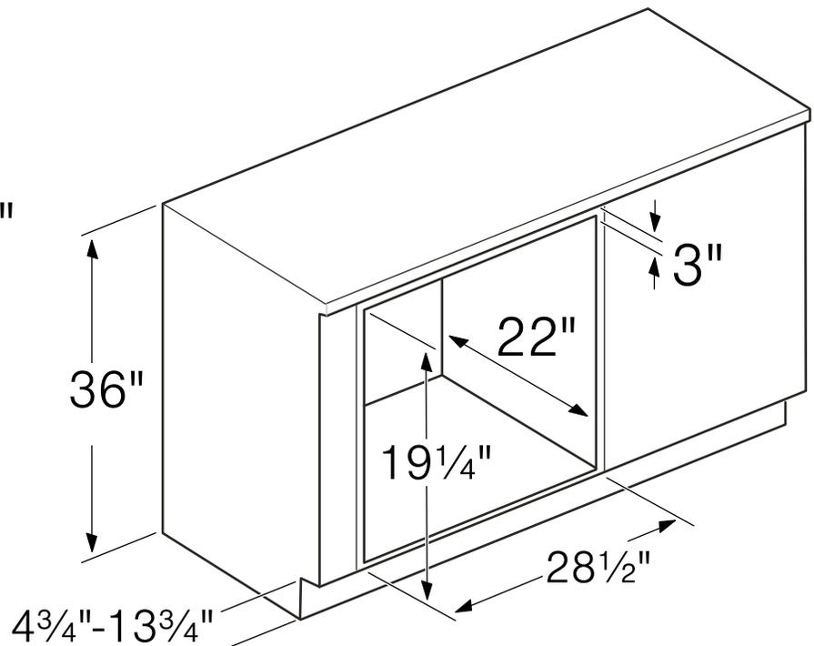
**NOTICE:** The cabinet base must be flat and capable of supporting a weight of at least 142 lbs (64.1 kg).
