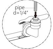
Put the blue clip back to the connector to lock the connection.
