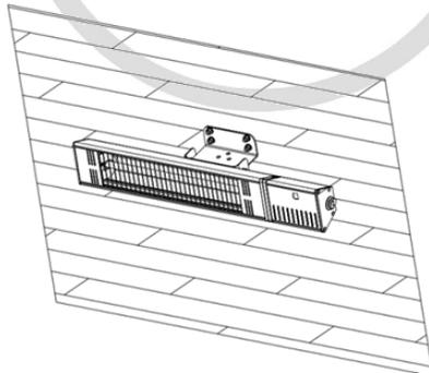
**Step 3:** Fix the mounting bracket over the four expansion bolts.
