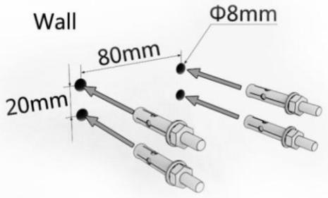
**Step 2:** Unscrew the four nuts, spring locks washers and plain washers from the four expansion bolts. Keep them for the next step.
