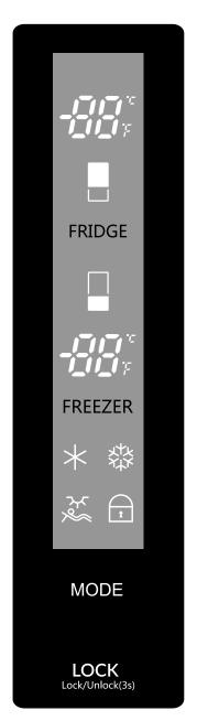
Default is Fahrenheit when power is on. Press "MODE" button 5 seconds, to switch between °C and °F. Other buttons use the same method to switch between two modes.
