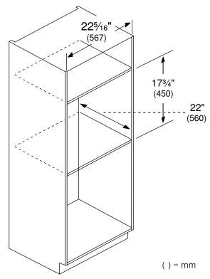
**NOTICE:** The cabinet base must be flat and capable of supporting a weight of at least 142 lbs (64.1 kg).
