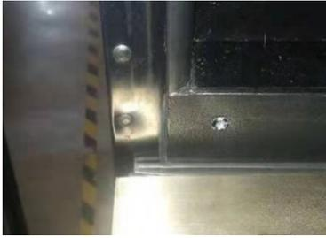
2. Take the lower hinge for left side from the accessory bag. Install it to the left side lower hinge position.
