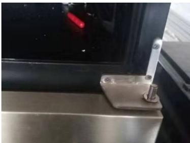
6. Unscrew and remove the lower hinge and door pin. Keep the hinge and pin in accessory bag for future use.
